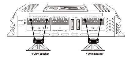
\*\*CAUTION! In the bridged mode, the amplifier must see a 4 Ohm load or higher. Any lower than 4 Ohms will cause the amplifier to overheat and possibly cause permanent damage to the amplifier!
